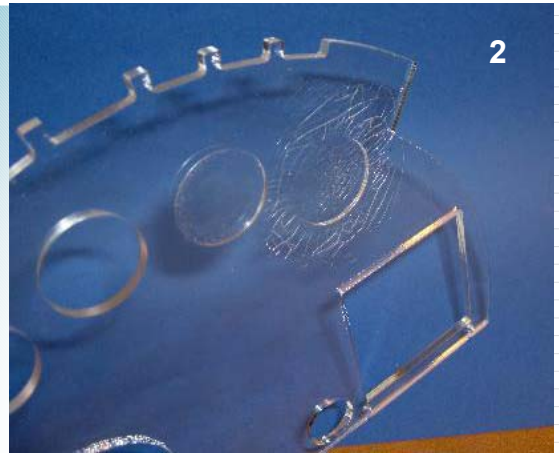
Photo 2 : Crazing of a piece of standard CN PMMA after forming, flame polishing and then spraying with a perfume diluent (right-hand part).
