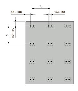
The tables are a non-binding aid. The proof of safety as well as an implementation planning based on it must always be provided in relation to the object. Influences from the hanger and horizontal profile are not considered. Maximum spacing from the vertical structure is 600mm.
