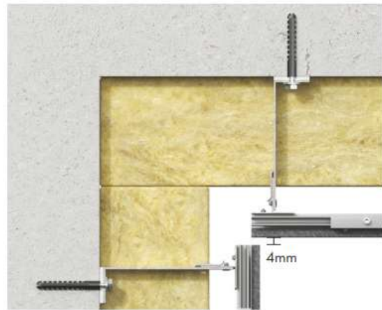
View: Internal corner with open joint
